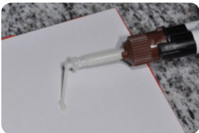
Fig. 10: Check of homogeneous mixing on the mixing block
