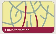
The double bonds contained in the resin matrix form chains during polymerisation of the monomers.
